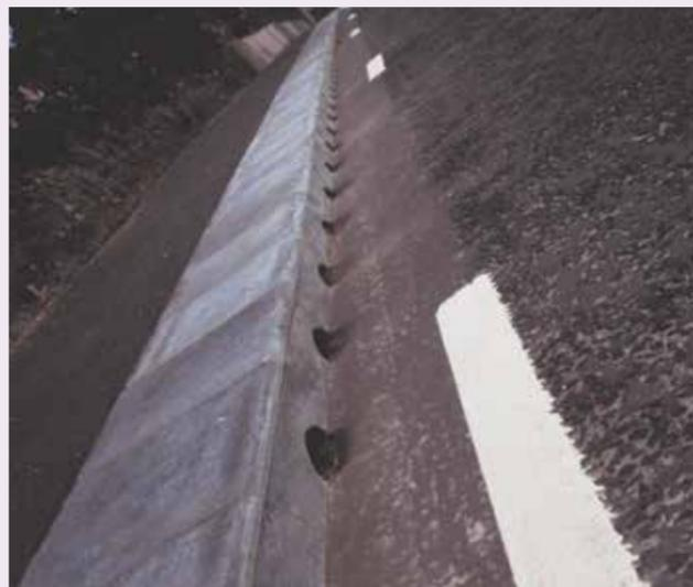
With its two-part high capacity channel base unit and soffit channel top unit, Highway dramatically reduces the need for expensive underground pipework along with the cost of excavation. Featuring inlet holes along the kerb line for fast and efficient water removal from the road surface, the channel stores and removes water to an outlet, eliminating the need for frequently placed outlet points.
