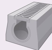
With its two-part high capacity channel base unit and soffit channel top unit, Highway dramatically reduces the need for expensive underground pipework along with the cost of excavation. Featuring inlet holes along the kerb line for fast and efficient water removal from the road surface, the channel stores and removes water to an outlet, eliminating the need for frequently placed outlet points.
